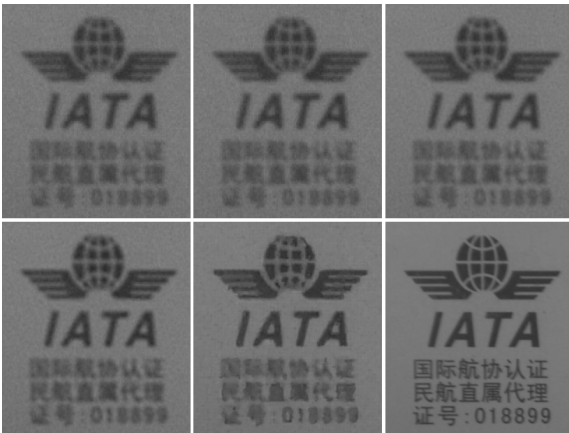
Figure 8. The SR results from eight LR images. From left to right, the top row is direct up-sampling, bicubic interpolation and the IBP result with PSF 1.5. The bottom row is the IBP result with ground truth PSF 2.5, our result and the original HR image.
