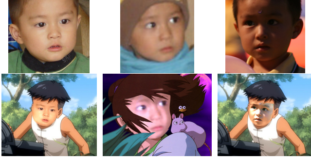
Figure 5: Example of results for bad face candidates. Upper row: selected faces; bottom row: synthesized images. From left to right: artifact caused due to wrong pose, too small resolution, and serious darkness of the selected face.
